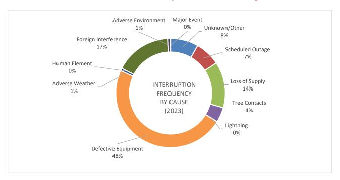
The above pie chart answers the following question: when power to a customer is interrupted, what's the likelihood of a given cause? **Note:** the above includes the cause "Loss of Supply", however this parameter is not within GSHI's control.
